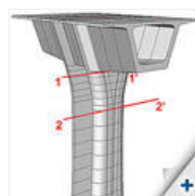
Location of sections for check of piers
