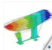
Scia Engineer - Eigenform Harbour House Antwerpen (in Bearbeitung)
