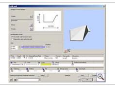
First, you have to use the 2D functions to draw the section of the cornice or parapet. After that you have to convert the section to a symbol.
