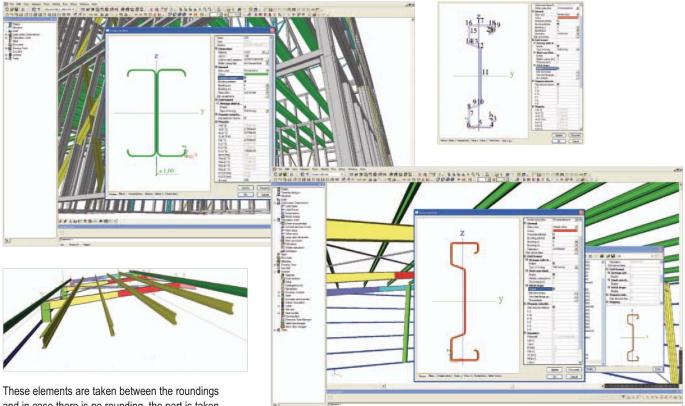
These elements are taken between the roundings and in case there is no rounding, the part is taken between the crossing points of the centre lines. The generated initial shape can be viewed and modified by the user.
